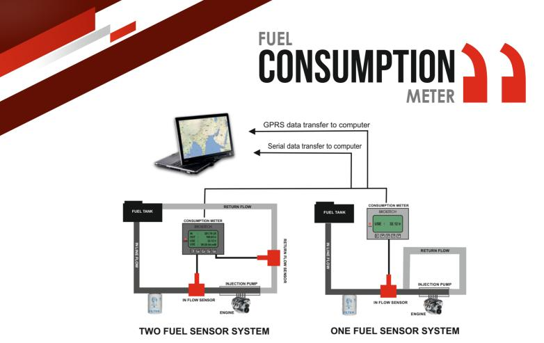
**BROILTECH** launched offline fuel consumption meter for vehicle and diesel generator fuel management, FCM is combination of two fuel flow sensor (One for supply line and Second for return line) and fuel calculator, fuel
